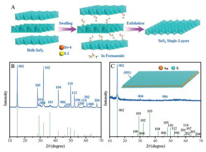
**Figure 1.** A) Exfoliation of hexagonal layered  $SnS_2$  into (001)-oriented freestanding  $SnS_2$  single-layers. XRD patterns for B) bulk  $SnS_2$  and C) (001)-oriented freestanding  $SnS_2$  single-layers.
