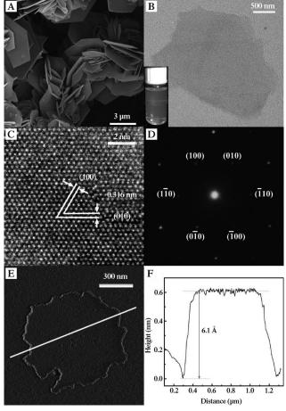
**Figure 2.** A) SEM image for bulk hexagonal  $SnS_2$ . Characterizations for (001)-oriented freestanding  $SnS_2$  single-layers. B) TEM image and the corresponding colloidal ethanol/water (1:1) dispersion displaying the Tyndall effect. C) HRTEM and D) the corresponding selected-area electron diffraction. E) AFM image and F) the corresponding height profile.
