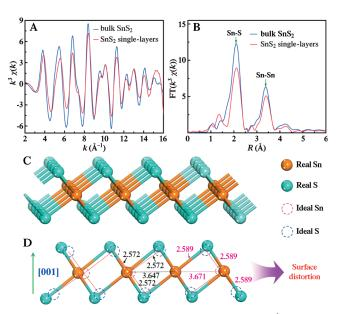
**Figure 4.** A) Sn K-edge extended XAFS oscillation function  $k^3\chi(k)$  and B) the corresponding Fourier transforms FT( $k^3\chi(k)$ ); k=wave vector and  $\chi(k)$  = oscillation as a function of the photoelectron wavenumber. C) Three-dimensional and D) two-dimensional structural models for SnS, single-layers.
